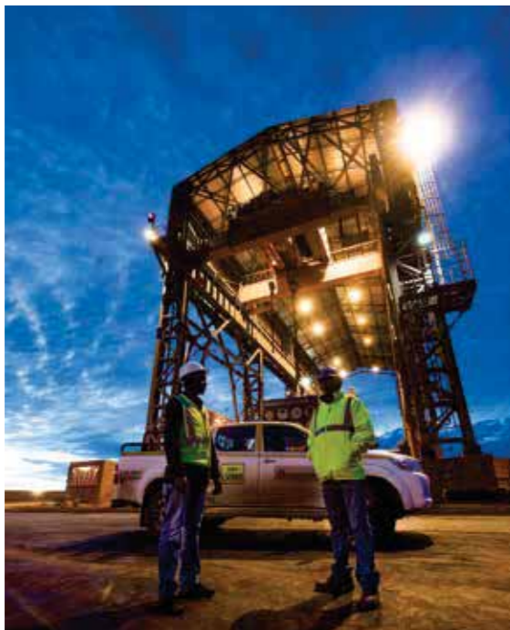
01 SHERQ officers Judge Thhaolagomo and Lantley Willems at the primary crusher at Kolomela mine. The mine has a production capacity of 10Mtpa and produces direct-shipping ore for the export market.
